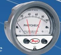
functions as versatile, highly repeatable pressure switches combined with a precise pressure gauge employing the time-proven Magnehelic gauge design. The Photohelic switch/gauge measures and controls positive, negative or differential pressures of air and compatible gases. Two phototransistor actuated, DPDT relays are included for low/high limit control.
