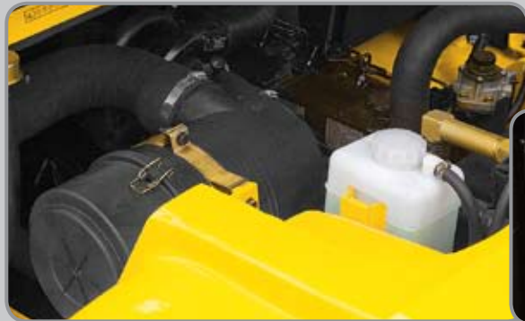
Easy change air cleaner The air filter is readily accessible for cleaning or replacement.
