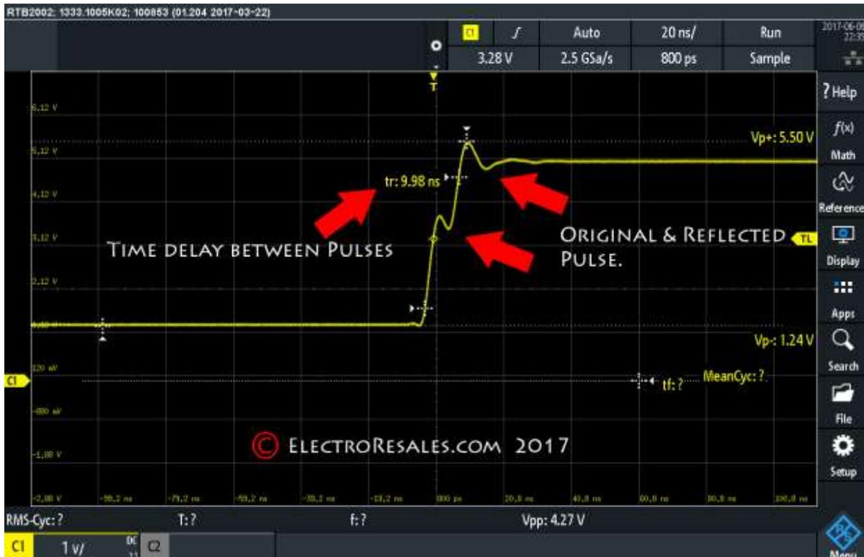
This image shows the original and reflected pulse on the scope screen, also as the scope used for these measurements had an auto measure option, the delay in ns is also displayed, your scope may not have this feature or may use user selected cursors to measure time or voltage. If no measuring method is available the time delay can be determined by counting the divisions or parts of divisions, between the two pulses.
