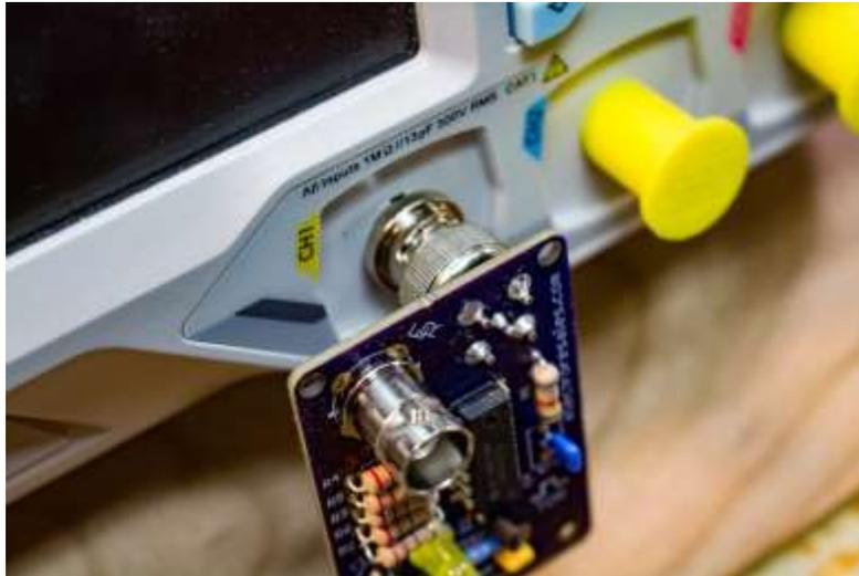
When the TDR is connected apply DC power, the LED should light, indicating the board is powered up. Once this is achieved, adjust your scope controls to display a square wave, exact settings will depend on your particular scope, however, aim to achieve the display shown in the next picture.
