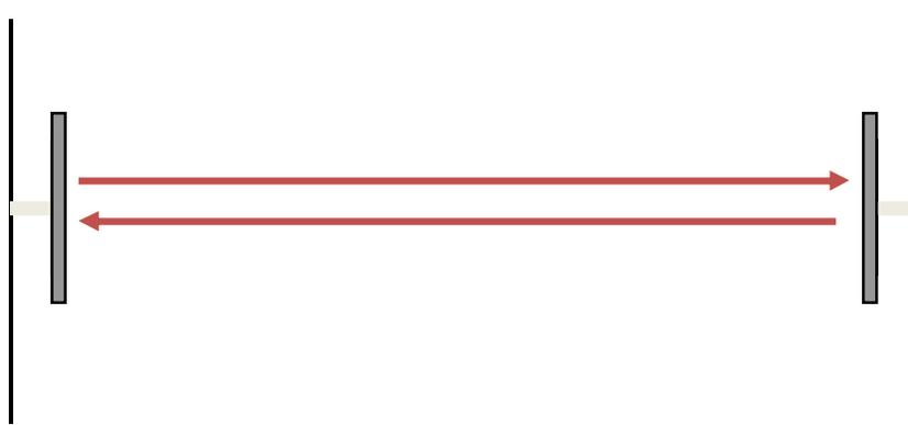
**To increase the sensitivity to carbon, the signal can be reflected back and forth many times.**
