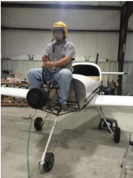
Jason Structurally Testing the Motor Mount
