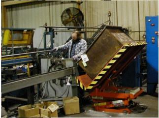
was required to incrementally adjust both vertical position and degree of tilt of a work platform to ergonomically "fit" a wide variety of employee heights and reaches – dramatically reducing bending and reaching motions associated with component part retrieval during the assembly process.
