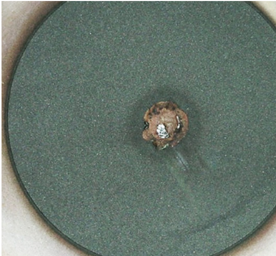
Fig.7 Another example of excessive power density. This was a high power water-cooled disc. The spot size must be increased to prevent this type of damage.
