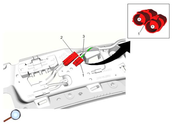
15. Separate connector #1 and connector #2 and insert the bypass harness supplied in the HMI kit.
