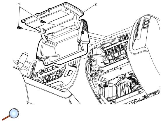
9. Remove the instrument panel upper compartment bolts (1). **Tighten**
