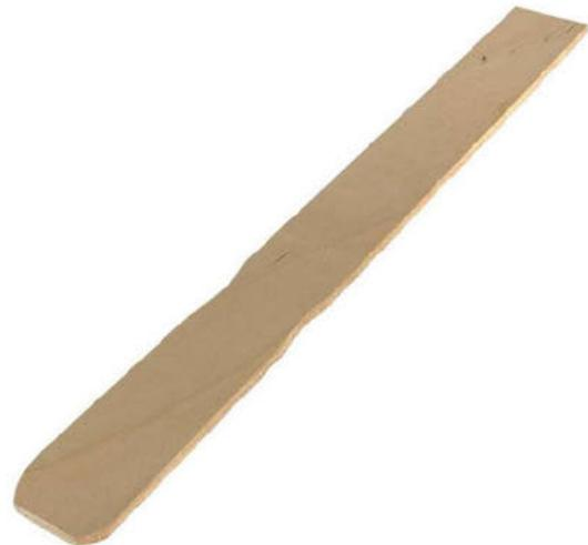
To use it, remove the gas cap (and the screen in the filler neck, if the car has one) and just dip the stick straight down until you touch the bottom of the gas tank. Now lift it out and see where the wet gas level is on the gauge. It will be approximate, but close enough to drive with some confidence, knowing you will have enough fuel.
