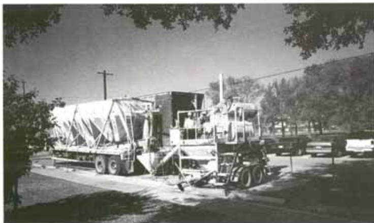
All photos courtesy of Karl Schack. Typical batching equipment and cement silo.
