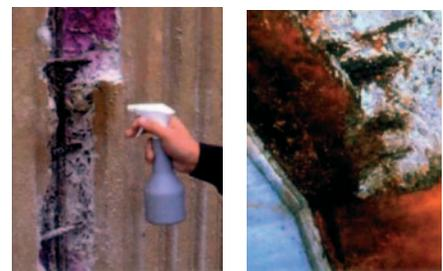
Carbonation testing of reinforced concrete.
