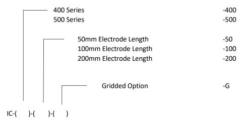
For example, an ion chamber 400 series with a 50mm Electrode length, with the gridded option would be denoted by: IC-400-50-G
