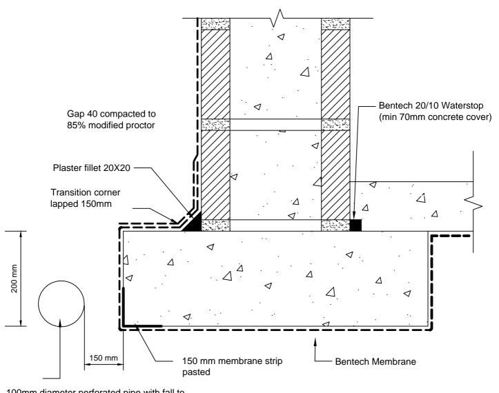
100mm diameter perforated pipe with fall to stormwater outlet.
