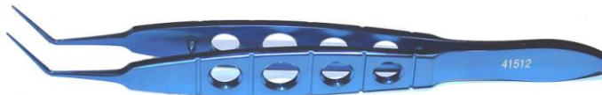
Notched Implantation Forceps 41512 Angled 0.25mm notched, shafts angled 45 degree, with 9.0mm platform, 108mm long
