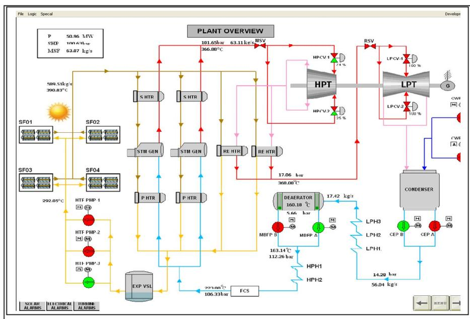
Closed loop controls, interlocks and permissives etc. have been considered for all important equipment. Some important closed loop controls include heat transfer fluid outlet temperature, steam generator drum level, condenser hot well level and Turbine Electro hydraulic control system.
