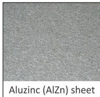
a. The cabinet is fabricated out of Aluzinc (AlZn) sheet to get the best possible conduction of the electromagnetic fields.
