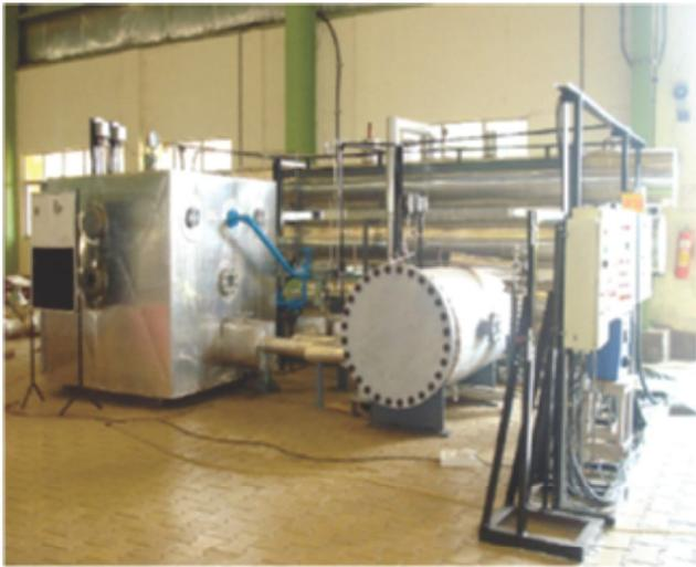
Figure-3: LOCA TEST CHAMBER
