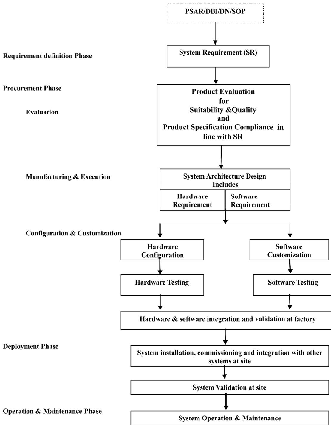
FIGURE-2: LIFE CYCLE FOR PRE-DEVELOPED SYSTEM (PDS)
