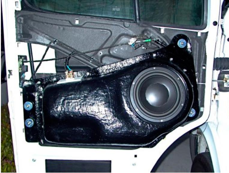
**Figure 21.** Finished door enclosure installation. The finished weight of each enclosure was about 35 lb (156 N).
