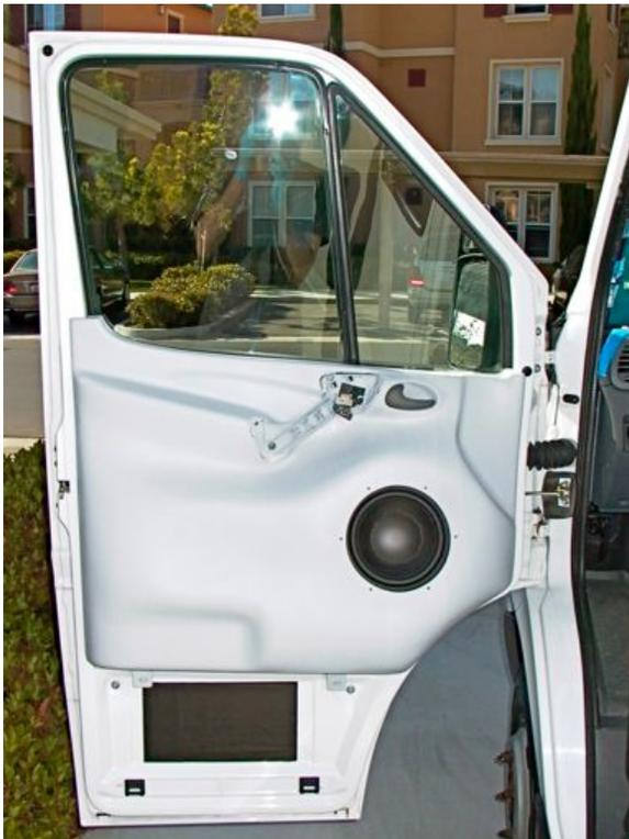
**Figure 32.** A two-component polyester high-build primer was sprayed onto the door panel. The primer was block-sanded with 320-grit sandpaper prior to the application of the color-matched, textured, two-component finish. While I did the sanding, Jorge Perez at Tri-City Paint (visit [www.tcpglobal.com](http://www.tcpglobal.com)) expertly sprayed the parts with primer and paint. If you live in the San Diego area, I highly recommend Jorge's work.
