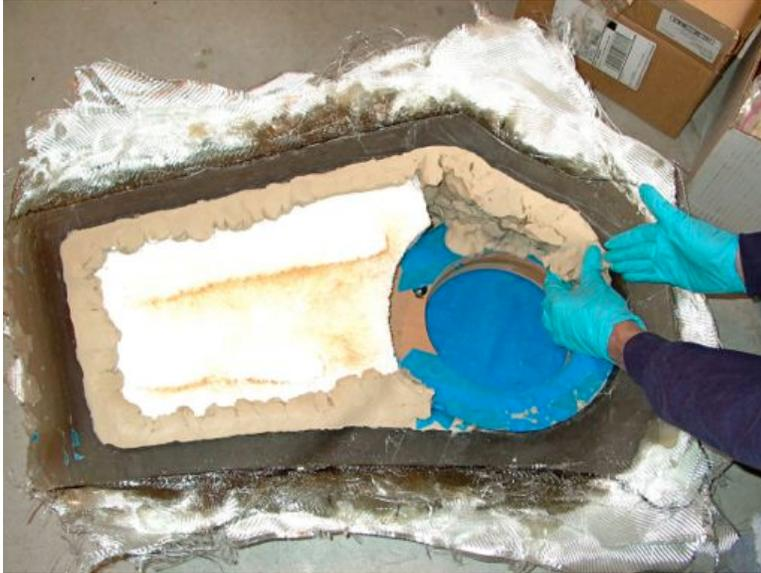
**Figure 13.** The KLEAN KLAY® and foam blocks were removed from the molded part. Notice the perfectly formed flange along the outside edge of the enclosure half. All fiberglass composite surfaces that were in contact with KLEAN KLAY® and mold release were thoroughly cleaned with acetone to remove any traces of residue.
