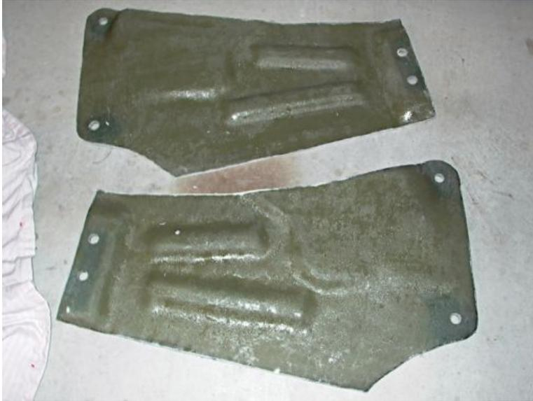
**Figure 3.** The door enclosures' back panels were formed from fiberglass composite comprised of woven roving. The complex curvature and ribs were intended to increase stiffness. The four mounting holes accommodated the rubber isolators.
