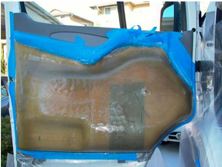
**Figure 24.** Blue masking tape and clear plastic sheet was used to protect surfaces from errant resin. The first four to six layers of fiberglass composite, comprised solely of 8.8 oz. twill woven roving and polyester laminating resin, were applied on the door mold and allowed to cure overnight.
