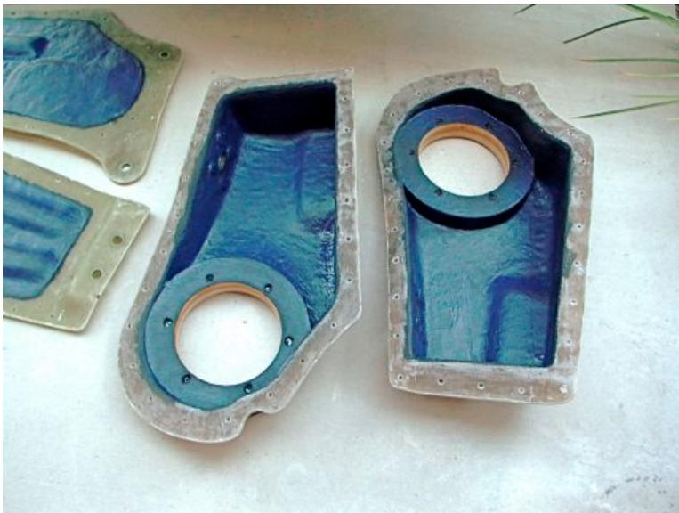
Figure 18. Ten successive applications of Cascade Audio's VB-1X were applied to the interior surfaces of the enclosures' front and back panels.
