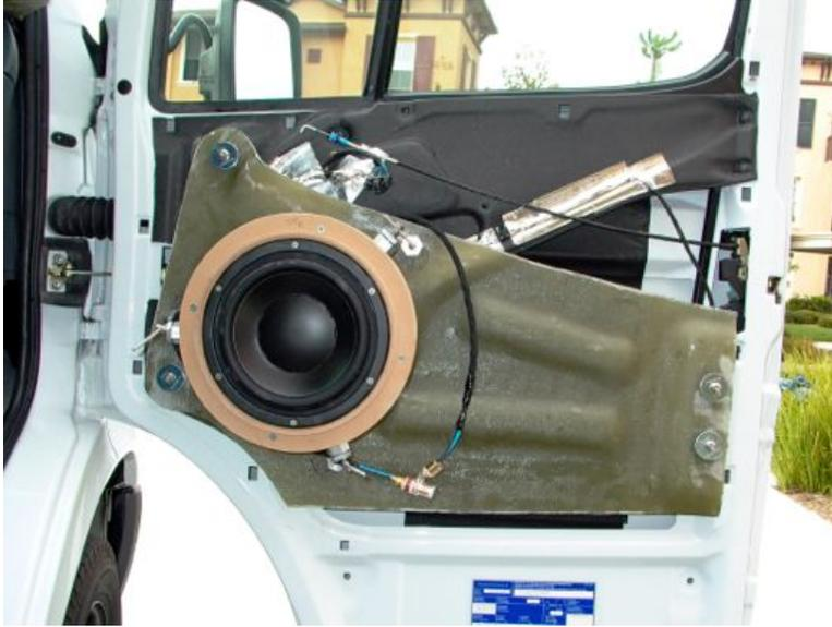
**Figure 5.** With the back panel mounted in its rubber isolation system, the loudspeaker transducer was appropriately aimed using my proprietary articulating mounting fixtures. Cascade Audio's VB-2 damper was applied to the inner door "skin", while several layers of Cascade Audio's VMAX was applied to the inner surface of the outer door skin.
