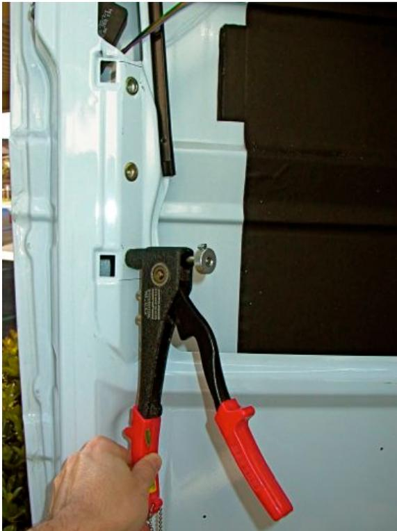
**Figure 2.** Five M8 x 1.25 rivet nuts were installed in each door. The pullout strength of each rivet nut was 15.7 kN (3,522 lb).
