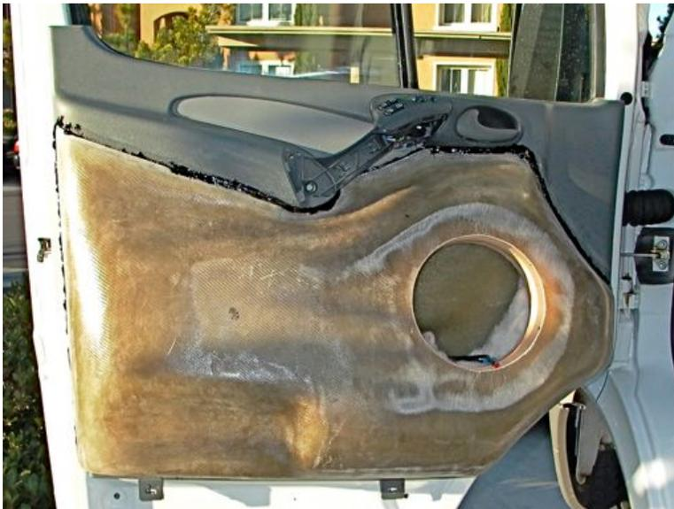
**Figure 28.** The factory door panel, comprised of a PP/EPDM copolymer, was sanded with 36-grit sandpaper and primed with 3M's Duramix™ TPO Adhesion Promoter. The fiberglass panel was bonded to the factory door panel using 3M's Duramix™ 4036 Thermoplastic Olefin TPO Repair adhesive. After the adhesive cured for 24 hours, the door panel assembly was removed and a liberal fillet of Duramix™ 4036 was applied to the inside of the bond line.
