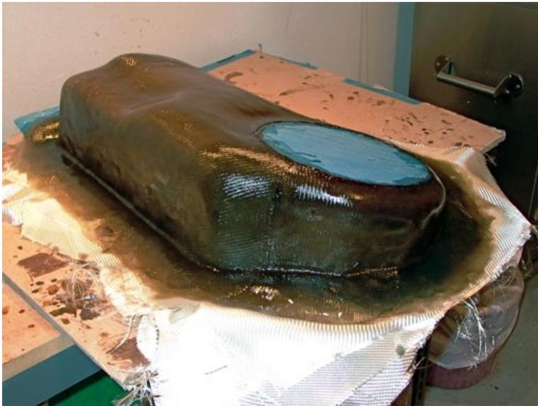
**Figure 12.** Numerous layers of fiberglass composite, comprised of 8.8 oz. twill woven roving and polyester laminating resin, were applied until the enclosure wall thickness reached about 12 mm (0.472 in), in accordance with the guidelines established in Part 5.
