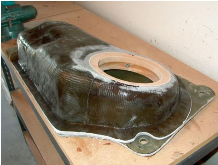
**Figure 14.** The edges of the front half of the enclosure were trimmed and sanded to match the edges of the back panel.
