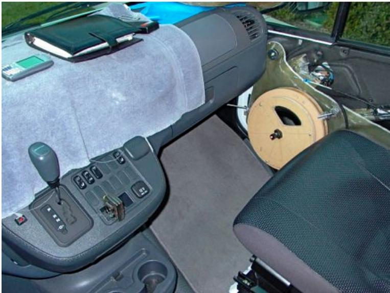
**Figure 6.** A magnetically attached jig, equipped with a laser gun sight, provided for precise aim. Notice the two red dots on the back edge of the tape measure, resting on the center console, were perfectly coincident.
