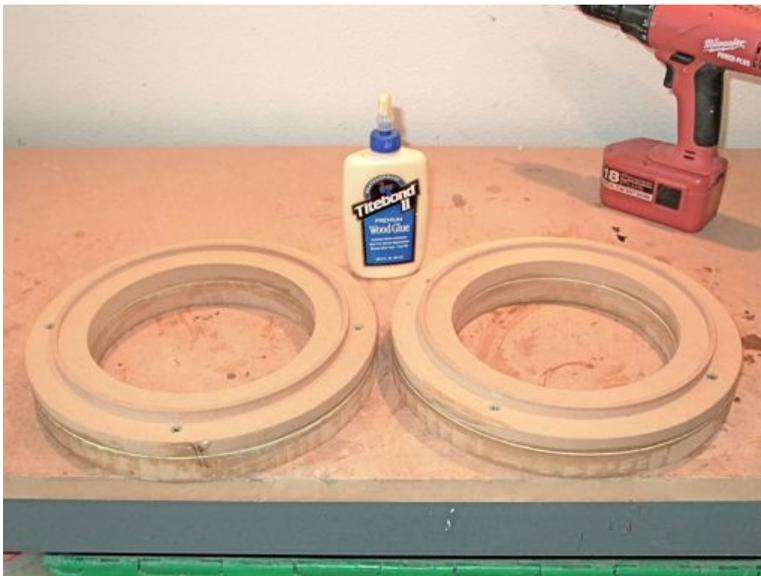
**Figure 4.** Loudspeaker transducer mounting rings were machined from 1-inch thick (nominal) MDF. An additional MDF ring was bonded to the machined rings to increase the overall thickness to 50.8 mm (2 in). M4 x 0.7 t-nuts were bonded to the backside of each ring, configured to match the loudspeaker transducer's bolt circle.
