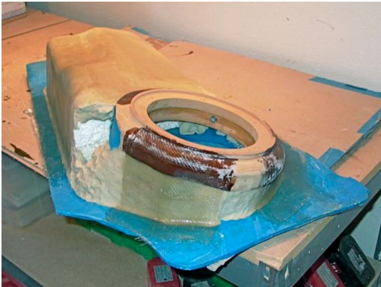
**Figure 10.** The first layers of fiberglass composite secured the MDF loudspeaker transducer mounting ring into position, enabling the mounting fixtures to be removed.
