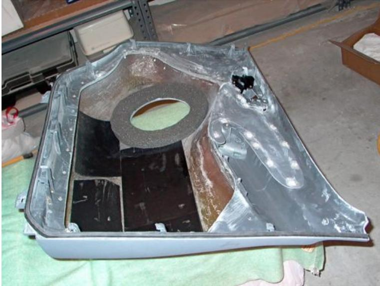
**Figure 33.** A ring of acoustical foam was applied to the inside of the door panel to act as a gasket between the door panel and the loudspeaker transducer. The gasket covers six M4 x 0.7 t-nuts, adhesively bonded to the inside of the door panel with Duramix™ 4040, configured to form the bolt circle for the loudspeaker transducer grill. Layers of VMAX were applied to the inner surface of the door panel.
