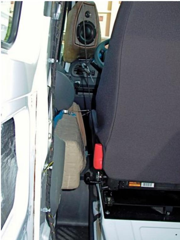
**Figure 8.** The driver's seat and seat swivel base restricted both the upward aim of the loudspeaker transducer and the protrusion of the enclosure into the cockpit area. Sufficient clearance to all objects was required in order to allow appropriate clearance for the door panel.
