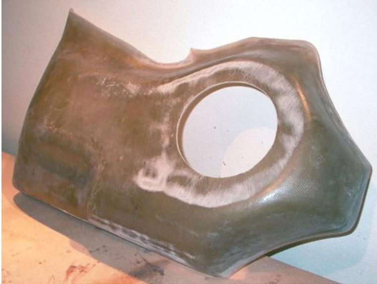
**Figure 27.** The edges of the panel were carefully cut to match the contours of the factory door panel. The hole for the loudspeaker transducer was also cut.
