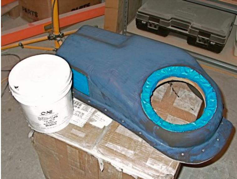
**Figure 19.** Seven successive applications of Cascade Audio's VB-1X were applied to the exterior surfaces of the enclosures' front and back panels. The total thickness of VB-1X applied to the inside and outside surfaces of the enclosures was nearly equal to the thickness of the fiberglass composite substrate.
