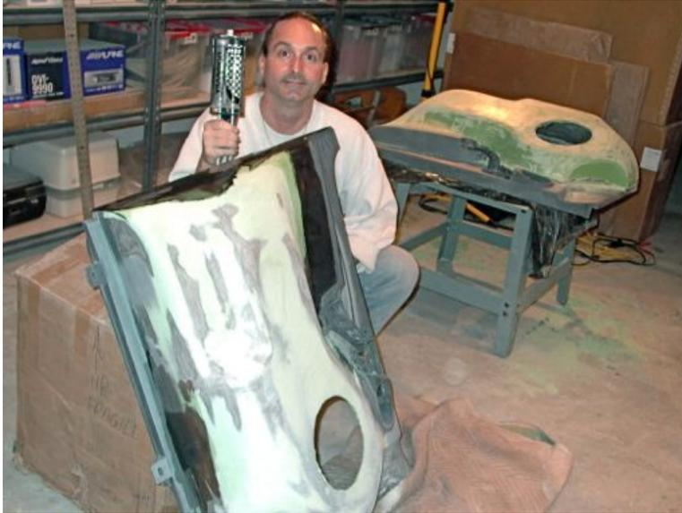
**Figure 31.** The fiberglass composite panel was filled and contoured with Evercoat®'s Rage Gold® body filler. 3M's Duramix™ 4058 E-Z Sand Plastic Finishing Paste was used to fill the transition from the PP/EPDM door panel to the fiberglass composite panel. The entire door panel was block-sanded with 80-grit sandpaper in preparation for primer.
