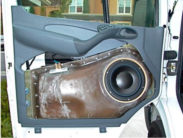
Figure 17. The MW180 loudspeaker transducer was installed in the enclosure for preliminary listening evaluation and tuning. The center of the factory door panel was cut away to make room for the enclosure.
