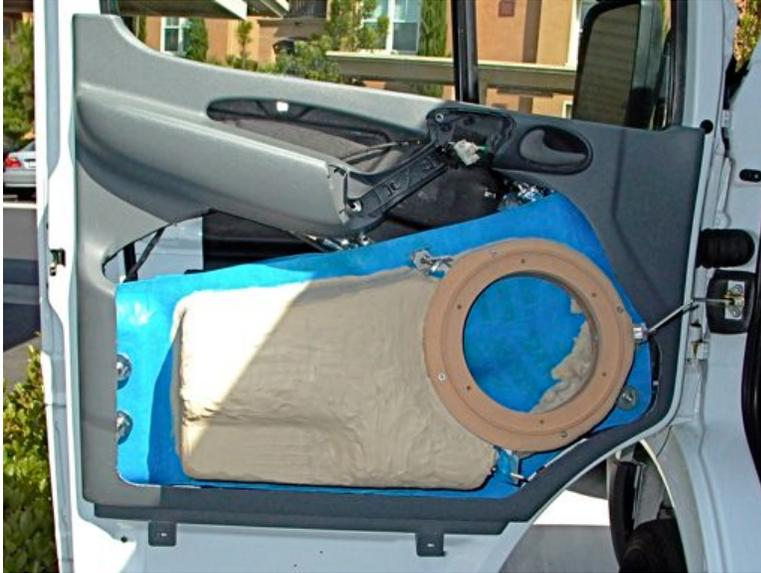
**Figure 7.** The mold for the front half of the enclosure was formed from foam blocks and KLEAN KLAY® (Art Chemical Products, visit <http://www.kleanklay.com>). The back panel and the MDF ring were protected with masking tape to prevent the absorption of clay residue.
