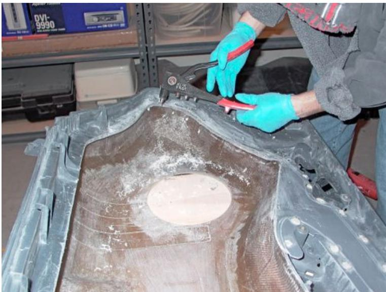
**Figure 30.** Aluminum peel rivets were installed to augment the adhesive bond with a mechanical bond.
