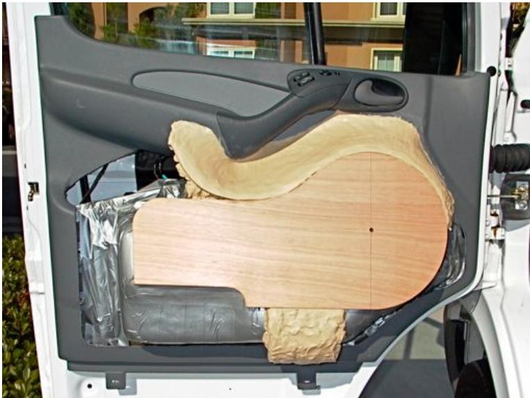
**Figure 22.** The mold for the new door panel was fashioned from plywood and KLEAN KLAY®. Duct tape was used to protect the underlying structures from KLEAN KLAY® residue.
