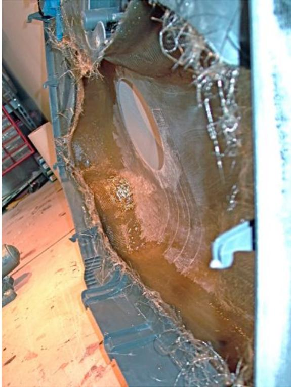
**Figure 29.** A substantial fiberglass composite gusset was added to bridge, and further reinforce, the bond between the factory door panel and the fiberglass composite door panel.
