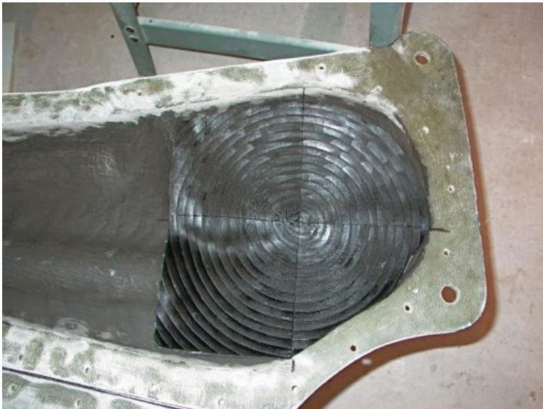
**Figure 20.** Cascade Audio's Deflex Power Pad was custom cut and bonded to the inside surface of each back panel using cyanoacrylate gel adhesive.
