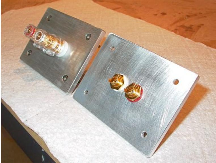
**Figure 15.** Binding post plates were machined from ¼-inch (6.35 mm) thick 6061-T6 aluminum, into which WBT binding posts were mounted.
