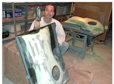
**Figure 31.** The fiberglass composite panel was filled and contoured with Evercoat®'s Rage Gold® body filler. 3M's Duramix<sup>™</sup> 4058 E-Z Sand Plastic Finishing Paste was used to fill the transition from the PP/EPDM door panel to the fiberglass composite panel. The entire door panel was block-sanded with 80-grit sandpaper in preparation for primer.
