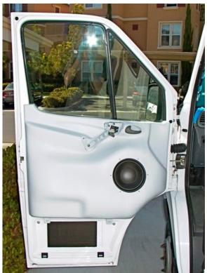
**Figure 32.** A two-component polyester high-build primer was sprayed onto the door panel. The primer was block-sanded with 320-grit sandpaper prior to the application of the color-matched, textured, two-component finish. While I did the sanding, Jorge Perez at Tri-City Paint (visit <u>www.tcpglobal.com</u>) expertly sprayed the parts with primer and paint. If you live in the San Diego area, I highly recommend Jorge's work.
