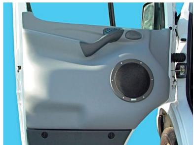
**Figure 34.** View of the finished door panel with Dynaudio's MW180 speaker grill installed. The total added weight of the isolated, highly damped, rigid, loudspeaker enclosure and door panel was about 50 lb (222 N)!
