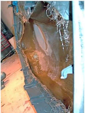
**Figure 29.** A substantial fiberglass composite gusset was added to bridge, and further reinforce, the bond between the factory door panel and the fiberglass composite door panel.
