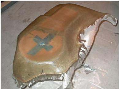
**Figure 26.** Additional layers of fiberglass composite, comprised of 8.8 oz. twill woven roving and polyester laminating resin, were applied to the molded panel until the thickness reached at least 6 mm (0.236 in).
