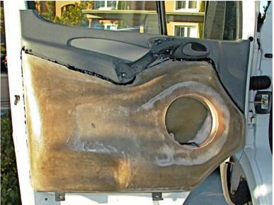
**Figure 28.** The factory door panel, comprised of a PP/EPDM copolymer, was sanded with 36grit sandpaper and primed with 3M's Duramix<sup>™</sup> TPO Adhesion Promoter. The fiberglass panel was bonded to the factory door panel using 3M's Duramix<sup>™</sup> 4036 Thermoplastic Olefin TPO Repair adhesive. After the adhesive cured for 24 hours, the door panel assembly was removed and a liberal fillet of Duramix<sup>™</sup> 4036 was applied to the inside of the bond line.
