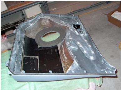
Figure 33. A ring of acoustical foam was applied to the inside of the door panel to act as a gasket between the door panel and the loudspeaker transducer. The gasket covers six M4 x 0.7 t-nuts, adhesively bonded to the inside of the door panel with Duramix<sup>TM</sup> 4040, configured to form the bolt circle for the loudspeaker transducer grill. Layers of VMAX were applied to the inner surface of the door panel.
