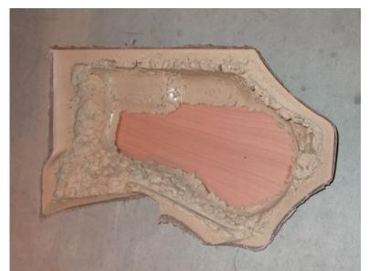
**Figure 25.** The molded door panel was removed from the door, but the mold came with it. The KLEAN KLAY® and the wood form were subsequently removed. KLEAN KLAY® residue was thoroughly removed using acetone. The inside surface of the molded part was sanded with 36-grit sandpaper and again thoroughly cleaned with acetone.
