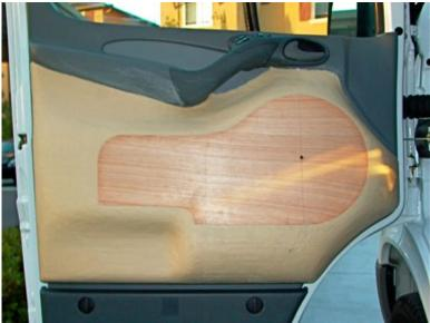
Figure 23. The finished door panel mold was liberally coated with mold release.
