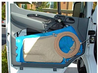
**Figure 7.** The mold for the front half of the enclosure was formed from foam blocks and KLEAN KLAY® (Art Chemical Products, visit <u>http://www.kleanklay.com</u>). The back panel and the MDF ring were protected with masking tape to prevent the absorption of clay residue.
