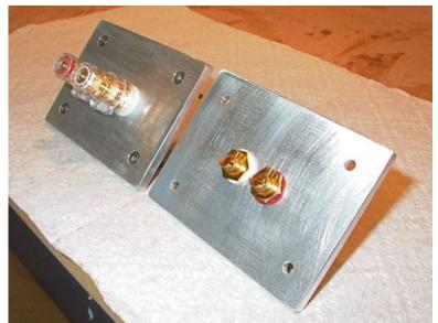
**Figure 15.** Binding post plates were machined from <sup>1</sup>/<sub>4</sub>-inch (6.35 mm) thick 6061-T6 aluminum, into which WBT binding posts were mounted.
