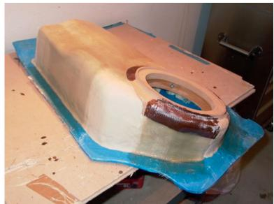
Figure 11. Additional KLEAN KLAY® was used to fill in the voids left by the mounting fixtures.
