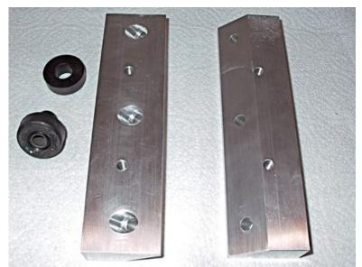
**Figure 1.** Aluminum brackets were machined and mounted to the rear edges of the doors to secure the rear edges of the door enclosures. One of the four rubber isolators is shown.
