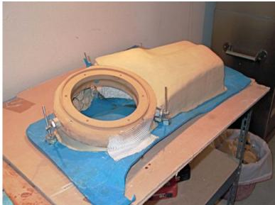
**Figure 9.** The MDF loudspeaker transducer mounting ring was appropriately shaped to accommodate layers of fiberglass composite. The mold was fashioned to allow room for a flange, which would allow the two molded halves to be bolted together. Liberal amounts of mold release were applied to the KLEAN KLAY® and masked surfaces.
