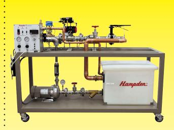
The Hampden **Model H-PVST-1** Pump and Valve System Trainer is a custom designed unit built to meet the plant specific training needs of the industrial facility. The trainer includes the basic facilities necessary to pump water (or other fluids) in a loop, together with the plant specific pump(s), valves and control configurations. Furthermore, all major components are flange fitted which allows easy removal from the unit. This will enable the trainee to learn the proper service procedures.
