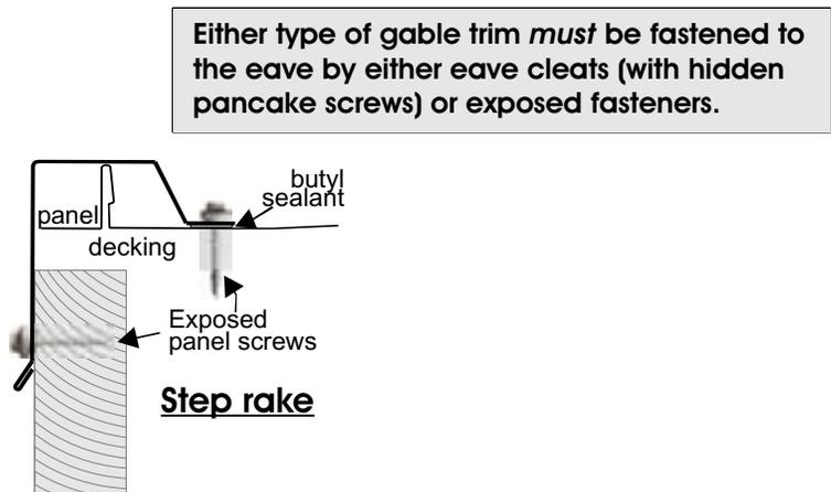
Either type of gable trim *must* be fastened to the eave by either eave cleats (with hidden pancake screws) or exposed fasteners.
