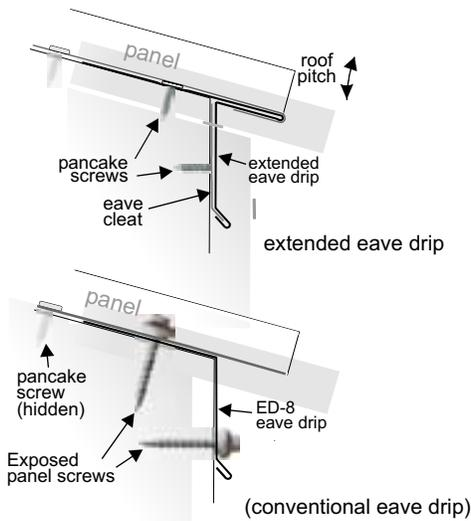
too steep). If more than one pitch is involved, specify the number of each pitch (drip edge comes in 10-foot lengths). Order 90 degree drip edge for square-cut eaves.
