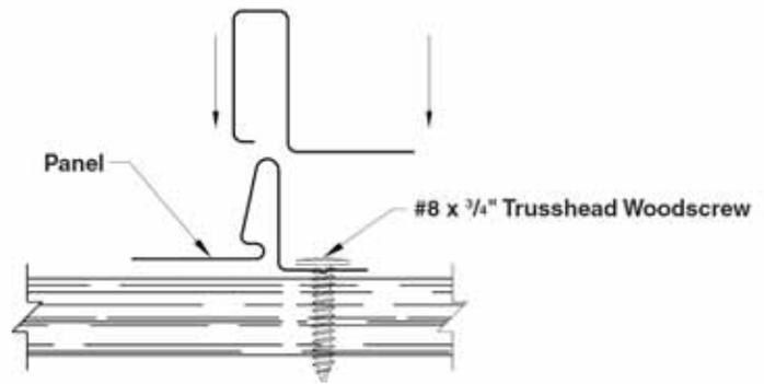
Standing Seam features approximately one-inch high ribs and a panel width of approx 16 inches. The "nail strip" and screws that attach each panel are in turn covered by each subsequent panel as each overlapping panel locks in place over the previous one.
