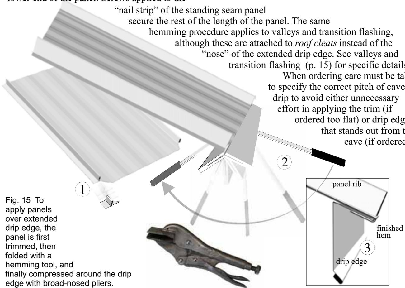
Fig. 15 To apply panels over extended drip edge, the panel is first trimmed, then folded with a hemming tool, and finally compressed around the drip edge with broad-nosed pliers.
