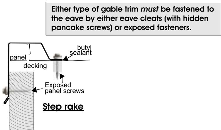
Either type of gable trim *must* be fastened to the eave by either eave cleats (with hidden pancake screws) or exposed fasteners.
