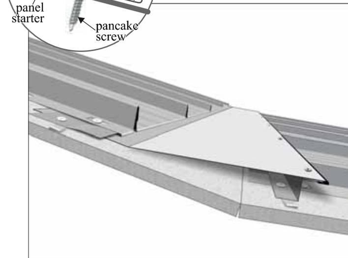
Fig. 21 Transition flashing combines the attachment techniques of valleys (top of page) with that used with ridge caps (p. 10). Notice the panel set-back that allows proper watershed from the upper panels onto the lower. The less the difference in pitch, as well as the flatter the roof, the greater the amount of set-back, and the more need for a longer lower side on the transition flashing.
