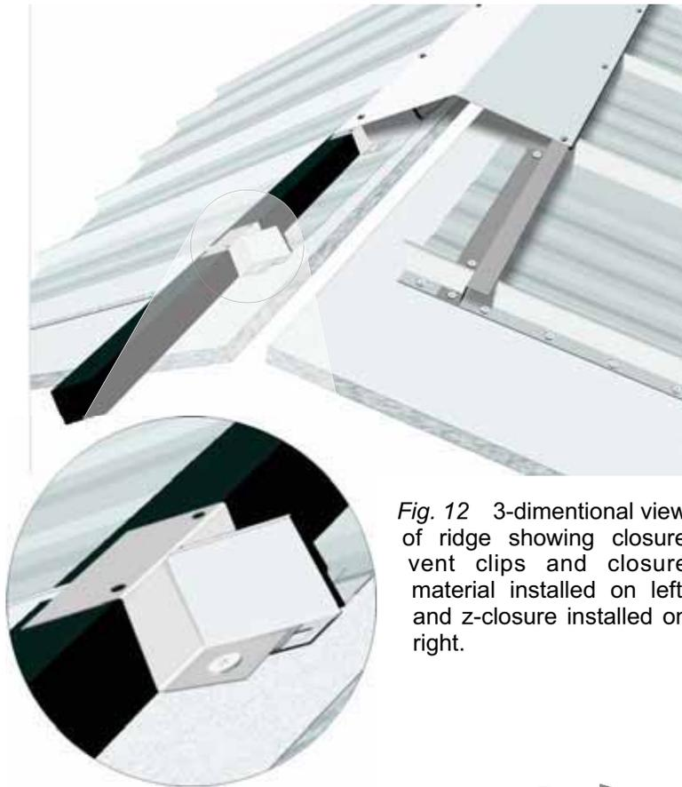
Fig. 12 3-dimensional view of ridge showing closure vent clips and closure material installed on left, and z-closure installed on right.
