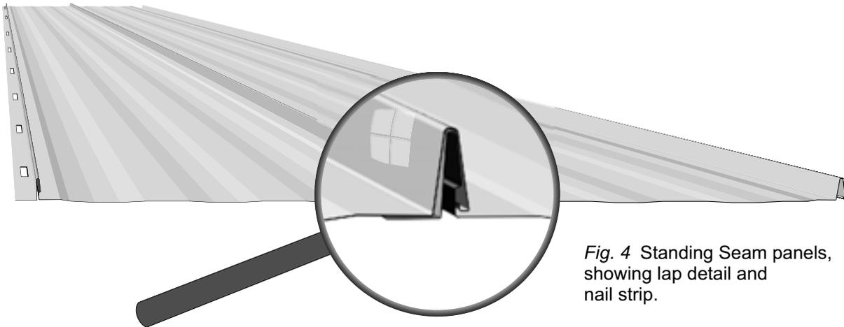
*Fig. 4* Standing Seam panels, showing lap detail and nail strip.
