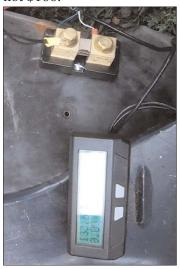
I also wanted to be able to get a read on the voltage pack digitally, and without closing the main contactor and making the vehicle live. I had an extra high current cycle analyst around (left, below meter shunt) that I wasn't using, and I wired that
