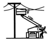
Maintain a clearance of at least 10 Feet (3 m) between any part of the machine or its load and any electrical line or apparatus carrying up to 50,000 volts. One foot additional clearance is required for every additional 30,000 volts or less.
