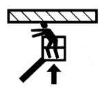
**Driving Crushing Hazard** Watch for obstructions around machine and overhead when driving.
