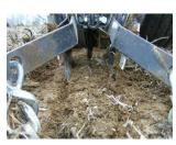
The Spading-Closing Wheel moves soil toward the seed at planting depth, while lifting and fracturing the surface layer to achieve compaction-free closing of the seed trench in wet, hard or sod conditions. With soil firmed around the seed from each side and the surface layer loosened, crops emerge sooner and planting can be done at the proper depth, even in wetter conditions, without fear of crushing the soil above the seed which would prevent emergence.
