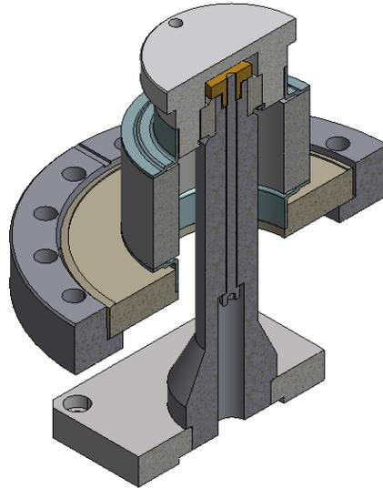
**Figure 2.** Cross-section view of ADC’s motion bellows assembly. The bottom plate of the bellows is mounted to the linear motion stack, the flange mounts to the vacuum chamber, and the top of the assembly is connected to the mirror base plate.
