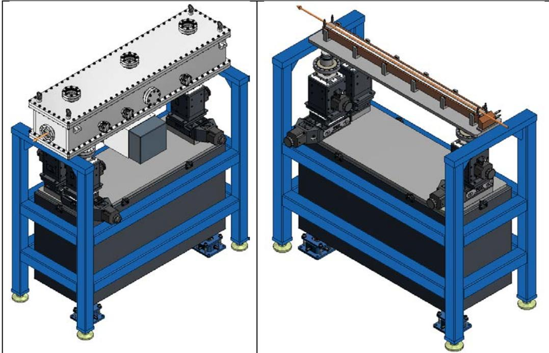
**Figure 1.** ADC Mirror System comprised of motorized stacked linear motions, granite plinth to support the motions, and UHV chamber mounted to steel framework. The steel frame is filled with sand to dampen floor vibrations. Kinematic feet below the granite plinth allow for adjustment of the mirror to its nominal position.
