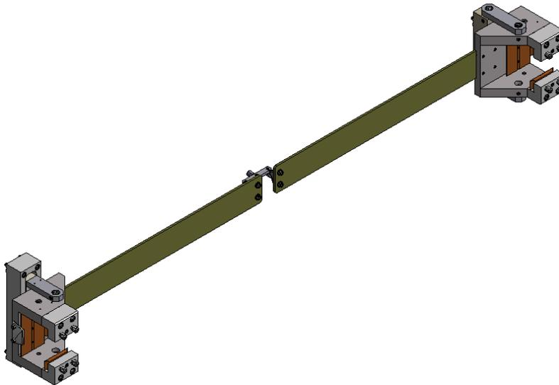
**Figure 4.** ADC's mirror bending mechanism. Each end of the mirror is held by pivoting clamps that are each attached to a leaf spring. Using a linear actuator and wiffle tree linkage, a displacement at the end of the leaf springs is used to impart a moment on each end clamp.
