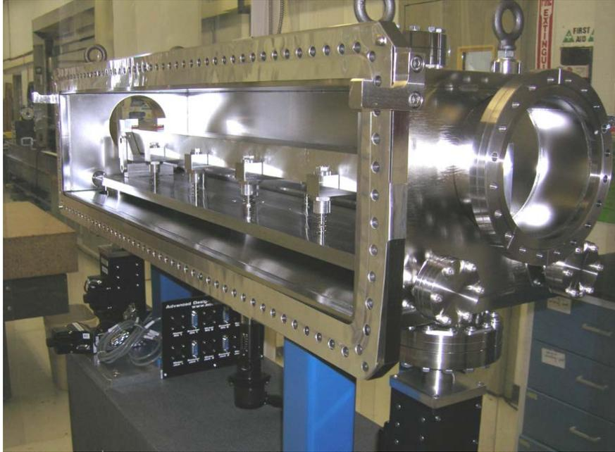
**Figure 5.** ADC vertical focusing mirror with bending mechanism, built for APS20-BM.
