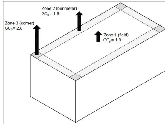
Illustration based upon ASCE 7-10, Fig. 30.4-2A ( $\theta \leq 7^\circ$ ); Effective wind area =  $10 \text{ ft}^2$
