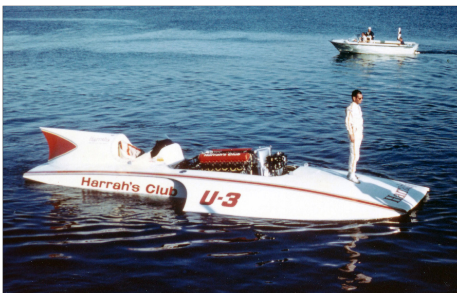
[Top] In 1968, the Harrah's Club was painted white due to Bill Harrah's superstitions, sported a pickle-fork bow, and a Rolls Griffon engine. [Above] The deep pickle-fork transformed into a blunt-nosed configuration by the time the campaign reached San Diego near the end of the season.
