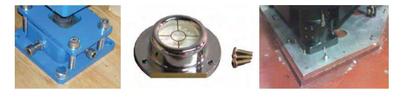
Permanent floor mounting options are also available with ADC optical tables. This is typically done by first grouting a precision flat plate to the facility floor. Before grout is poured, the plate is leveled and can be tied into the floor using threaded inserts. The grouted plate provides a permanent and extremely stable floor mount for the optical table.
