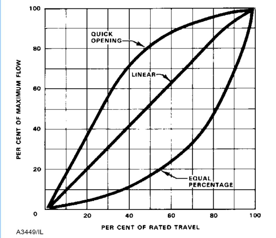
**Inherent Valve Characteristics**
