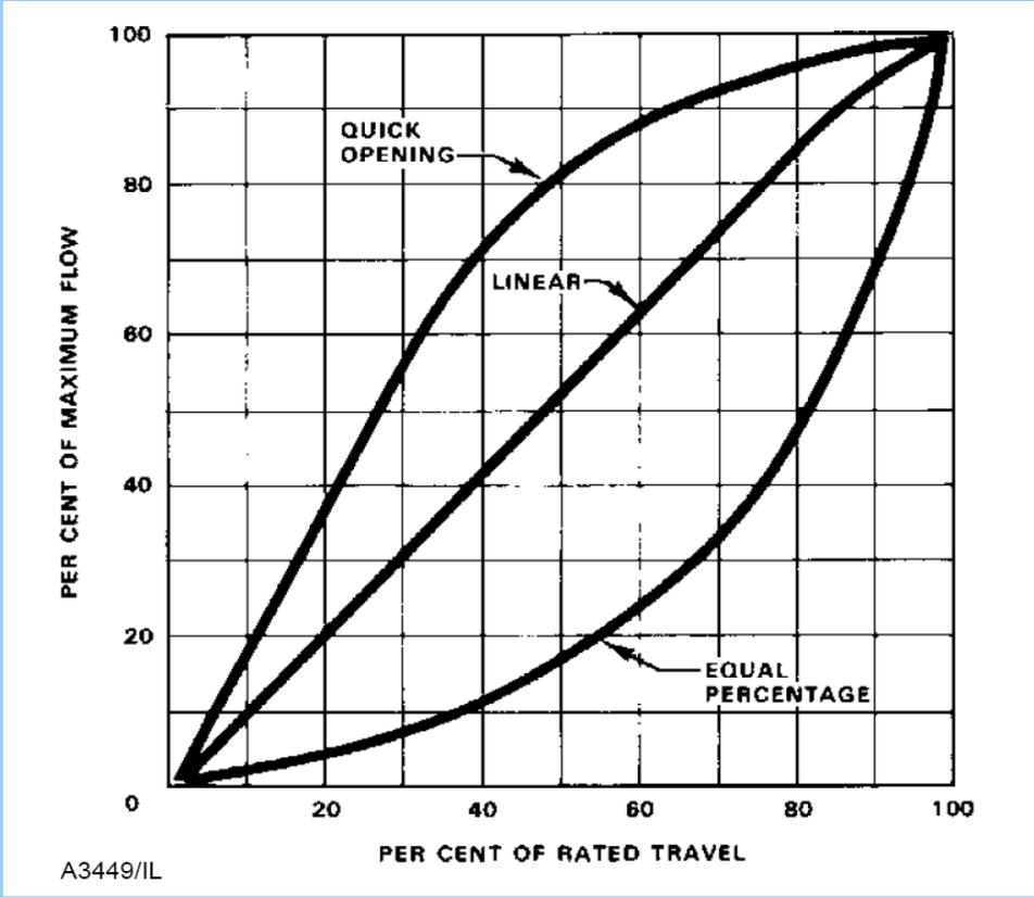
Inherent Valve Characteristics
