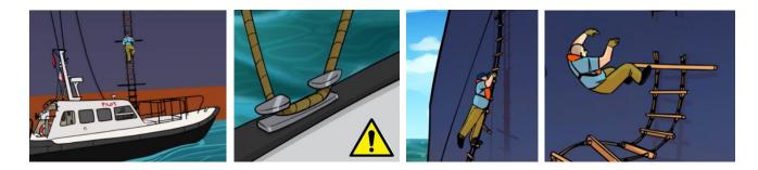
Retrieval lines must be rigged at or above the lower spreader and must lead forward so that the line does not risk becoming entangled with the pilot boat as it approaches from aft.
