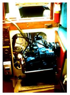
shaft log, and packing gland. The new engine encroached upon the cabin under the cabin ladder, the floor of that part of the cabin requiring reinforcing to a 'strong-back' rigidity to accommodate the forward engine mounts. After the old engine bed was removed, the new bed required a grinding away of all the old fiberglass and carefully exposing a clean glass hull upon which to adhere the new fiberglas component of the new bed. Not a small amount of labor - and potentially very costly!
