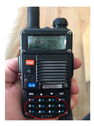
5. In order to talk press and hold the PPT button (PPT stands for "press to talk") while talking, and your on the air. While you are holding the PTT button you are transmitting. Hold the radio vertical, close to your mouth (1"), and at a slight angle to your face so you are not speaking directly into the radio. Press the PTT button around 1 second before speaking and for 1 second after. If possible, outdoors is much better. Note: the red call button toggles between FM radio and GMRS radio.
