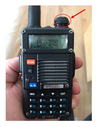
2. You can change between frequency mode and channel mode by pushing the red VFO/MR button on the face of the radio. Use frequency mode to input a desired frequency (see details in step 4). You can store favorite frequencies as channels, and access them in channel mode. Note, the channel number will not necessarily correspond to the numbers on other GRMS radios and our frequency chart unless you input them as such.
