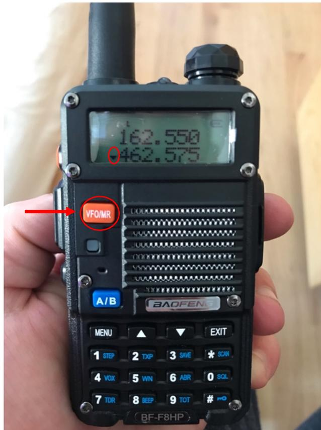
4. To enter a frequency to monitor/transmit on, make sure you are in frequency mode (toggle back and forth using the red VFO/MR button). After selecting the desired frequency on the display using the blue A/B button, you can edit it using the key pad. In order to input the GMRS channel 16 frequency of 462.5750 MHz (our priority frequency), you would use the key pad to enter “4” “6” “2” “5” “7” “5” “0”. This will immediately become the active frequency, and you are now ready to transmit/ receive.
