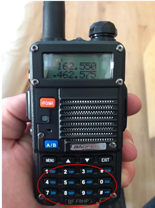
5. In order to talk press and hold the PPT button (PPT stands for “press to talk”) while talking, and you are on the air. While you are holding the PTT button you are transmitting. Hold the radio vertical, close to your mouth (1”), and at a slight angle to your face so you are not speaking directly into the radio. Press the PTT button around 1 second before speaking and for 1 second after. If possible, outdoors is much better. Note: the red call button toggles between FM radio and GMRS radio.
