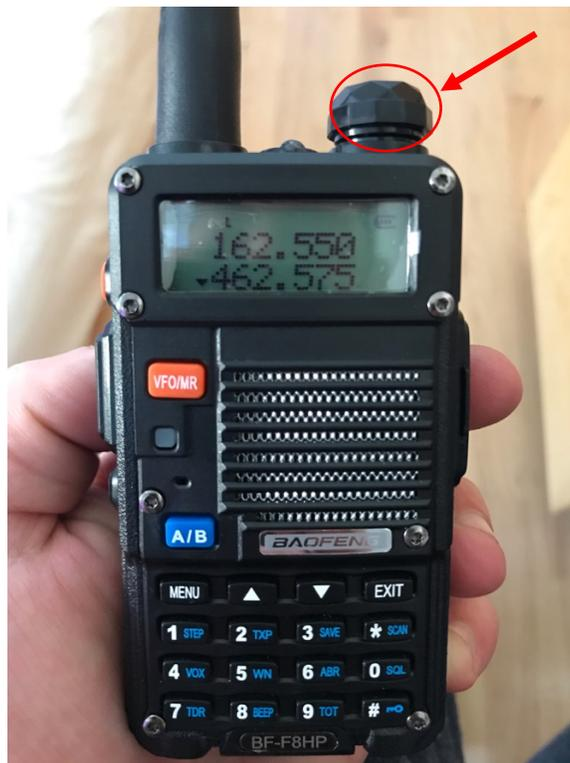
2. You can change between frequency mode and channel mode by pushing the red VFO/MR button on the face of the radio. Use frequency mode to input a desired frequency (see details in step 4). You can store favorite frequencies as channels, and access them in channel mode. Note, the channel number will not necessarily correspond to the numbers on other GRMS radios and our frequency chart unless you input them as such.
