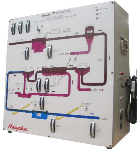
MODEL H-DWTS-CSI – Digital Wastewater Treatment Simulator
