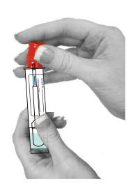
SNAP CAP firmly for transport. Place center of specimen seal on top of tube and press down both sides. Complete paperwork and send sample to laboratory.
