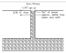
\*Note: Both maintenance types will be most effective when the joint aggregate material is filled to the "lip" of the paver. If the joint material has settled more than the joint width, plus 1/8 inch below the paver *lip, the maintenance* equipment is significantly less effective and potentially more expensive.
