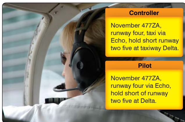
Figure 1-14. Example of taxi and “ hold short ” instructions from ATC to a pilot.
