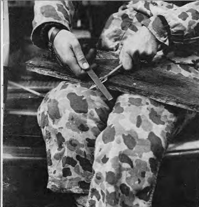
Here are two ways of sharpening broadheads. Crisp, downward strokes of a 6" mill file will give a rough, deadly edge to most heads. Some bowhunters prefer to hone blade on an oil stone. With most heads, filing is much easier
