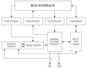
Fig.1: Block diagram of I2C Bus Interface
