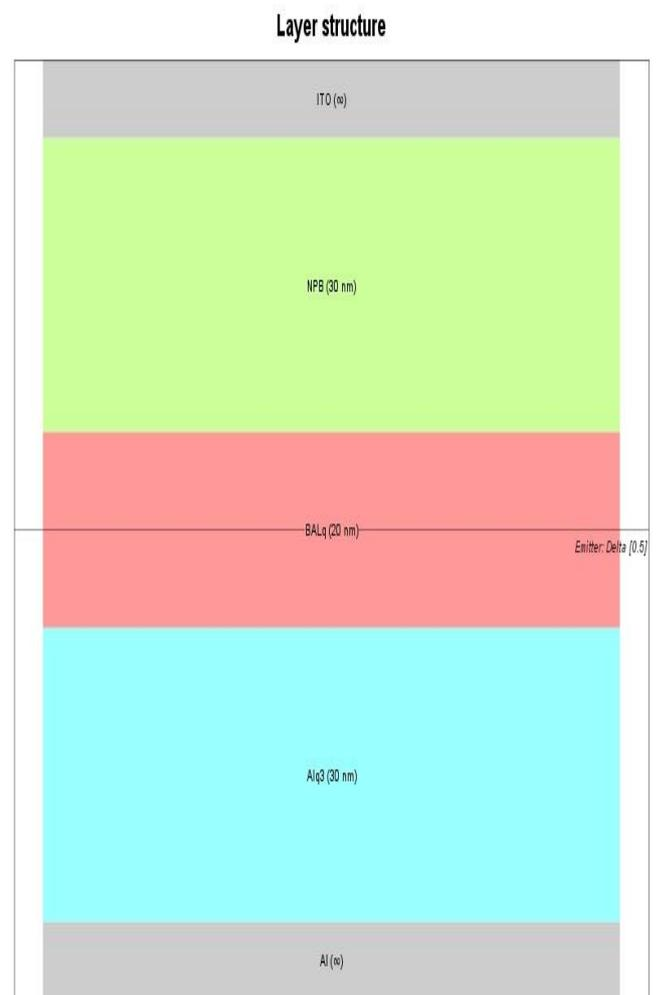
Fig. 2(a) Schematic diagram of Device A
