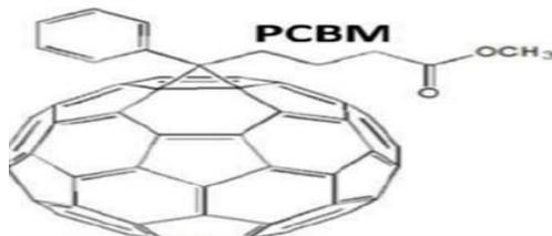
Fig. 2(c) Chemical structure of PCBM
