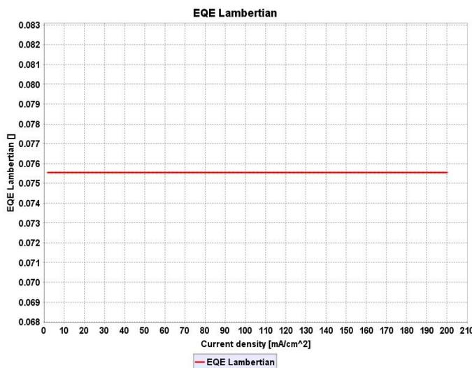
Fig. 3(c) Device A EQE Lambertian graph
