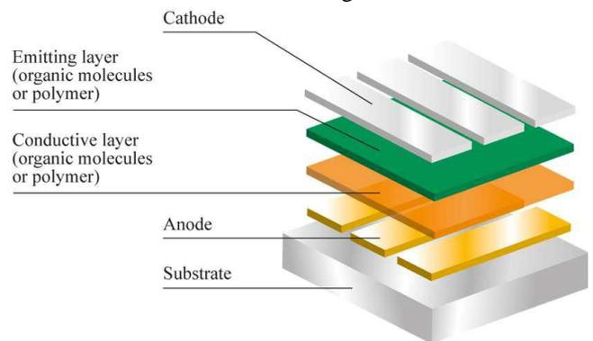
Fig. 1 Basic structure of OLED [3]
