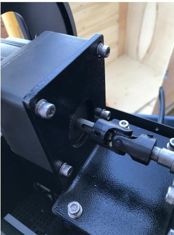
Loosen the 4 bolts that hold motor to mount and loosen couple set screws or bolts then remove motor and replace coupler. Next reassemble
