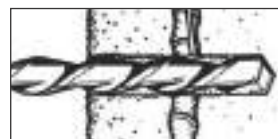
3. Return to hammer drilling to desired depth
