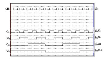
Fig 6: Data bits generated by counter
