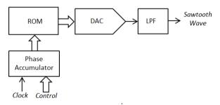
Fig 3: DDS based sawtooth generator
