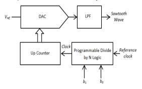
Fig 4: Proposed programmable sawtooth generator
