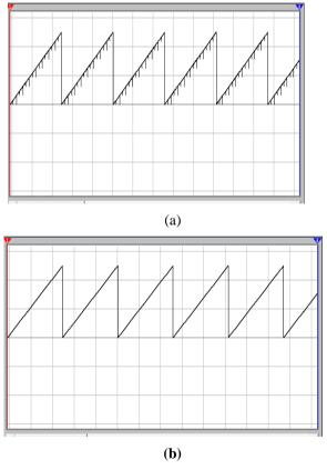
Fig 2: Waveform generated at the output of (a) DAC and (b) Filter
