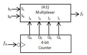
Fig 5: Programmable frequency divider
