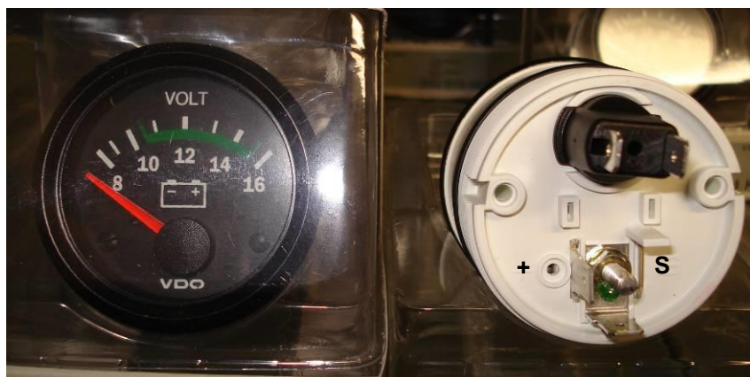
Figure 23. Voltage Gauge Connections
