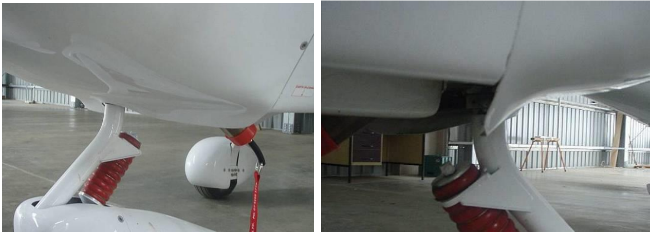
Figure 58: Lip to aid cooling as installed on a Jabiru.
