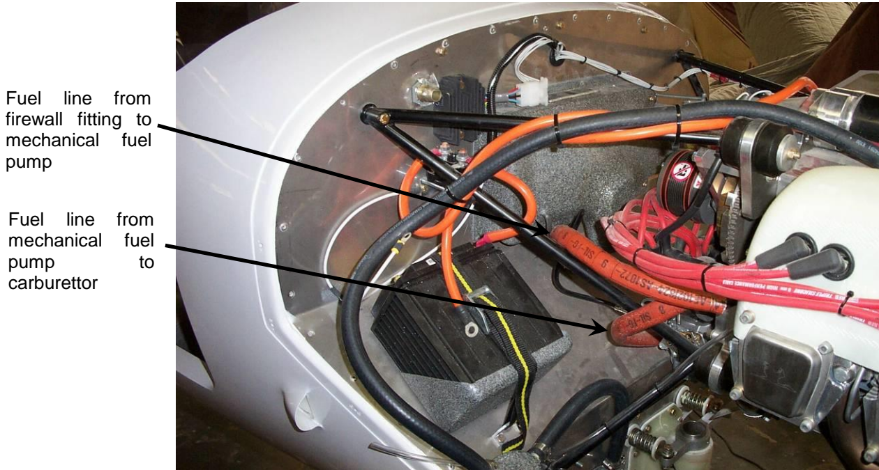
Figure 45. Fuel Connections General
