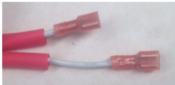
Figure 12 - Alternator leads must be of different lengths
