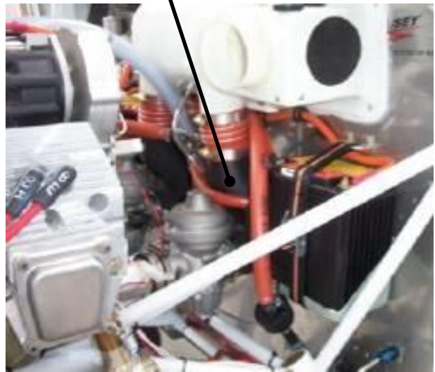
Figures 6 & 7. Typical Upper Engine Mount, Air Intake Installation
