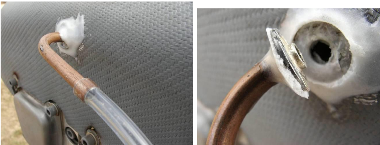
Figure 63: Ram Air duct pressure tapping.
