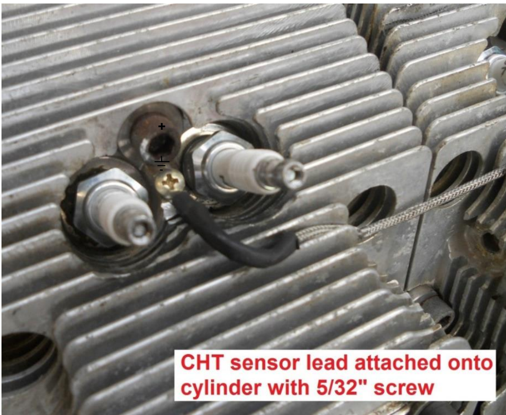
Figure 26. CHT sensor between plugs.
