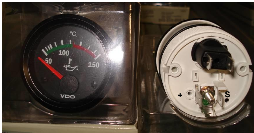
Figure 20. Oil Temperature Connections
