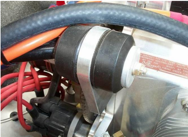
Figures 6 & 7. Typical Upper Engine Mount, Air Intake Installation
