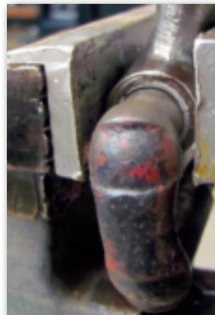
Test the fit of the spring shackle (hanger) in the new perch bushing and the job is done!
