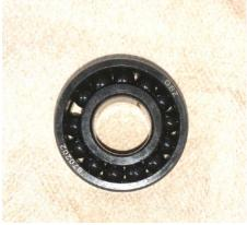
ONCE REMOVED REPLACE WITH NEW BEARING FOLLOWING REVERSE PROCEDURE AND PACK BEARING WITH FRESH NEW GREASE:
