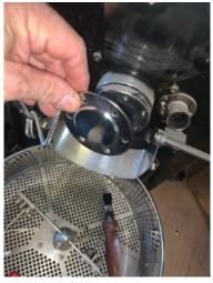
REMOVE INNER SHAFT BOLT AND WASHER:
