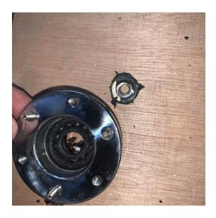
USING A WOOD DOWEL OR OTHER TOOL THAT FITS INSIDE BACK SIDE OF BEARING HOLDER TAP OLD BEARING OUT:
