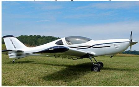
Lightning lives up to its name, running easily to the 120-knot maximum for LSA, especially when powered with a very muscular six-cylinder, 120 horsepower Jabiru 3300 powerplant. Every Lightning to date has been a tricycle gear airplane and, honestly, for most pilots, that is the right choice. However, like many aviators, I love the look of a tail dragger so when I stumbled across the one you see in the photos, I did a double take. Whoa! That looks hot!
