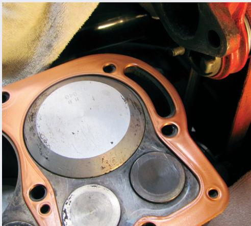
Set the cylinder head down (use of a handle is nice for the heavy iron head, or made easy with the newer, lighter aluminum high compression heads). Run down the bolts into the block. On the aluminum head, stainless steel washers go under the bolt head to prevent galling the aluminum when tightening the bolts. Use of anti-seize lube on the head bolt threads will make removing them later a bit easier with less risk of breaking.
