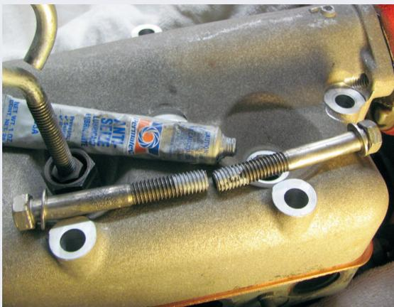
Finally, secure the bolts in the proper sequence. It's important to use a method in tightening so the head and gasket is squeezed from the center of the cylinder block to the outside, in a rotation. By tightening the center of the head first, then alternating the tightening of bolts to the outer edges, the cylinder head is best fitted, ensuring the gasket is flattened in center first. That is where the gasket is most narrow between the cylinders.
