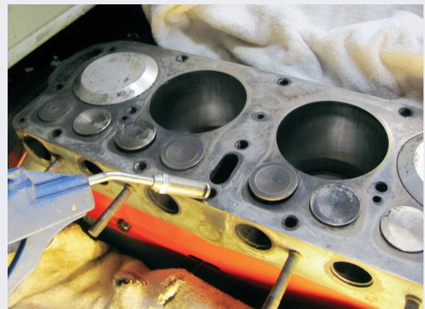
Next, the gasket is prepared. Using a copper-faced gasket, spray liberally with gasket sealer on both sides. Turn the engine over so #1 and #4 pistons are up, to help locate the gasket. Place the gasket correctly, as the Ford head gasket has the small opening at the front of the block. The larger water opening is at the rear of the block.
