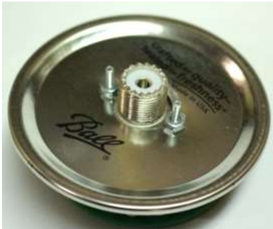
Lid plus load assembly mounted and bolted in place.
