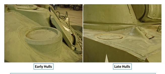
Mounting Locations for Mast Bases MP-37 and MP-57 when used with SCR-506 in Sherman Command Tanks
