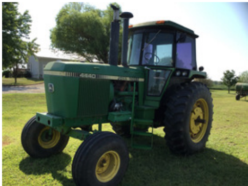
John Deere 4440, cab, air, triple hydraulics, 130 hp
